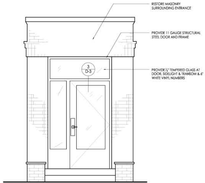
1 TYPICAL BUILDING ENTRANCE SCALE: 1/2" = 1'-0"
